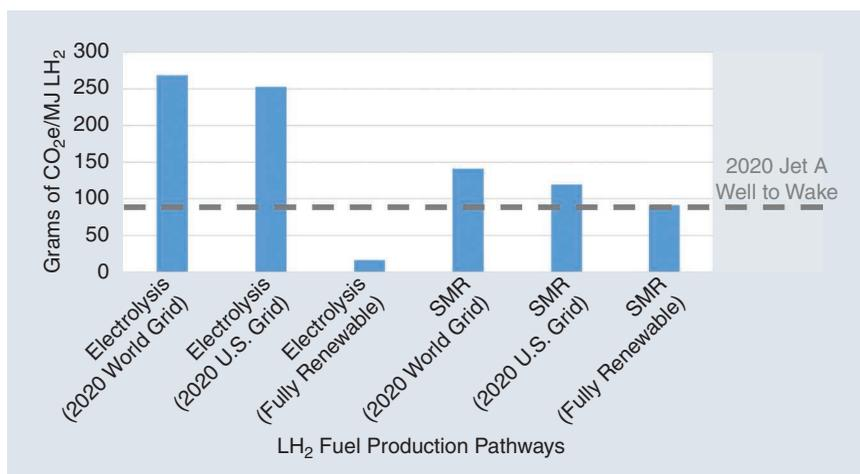
**Figure 6.** The CO<sub>2</sub>-equivalent (CO<sub>2</sub>e) lifecycle of LH<sub>2</sub> fuel production under different grid scenarios. SMR: steam methane reforming. (Source: Nicholas D. Applegate, Boeing; used with permission.)
