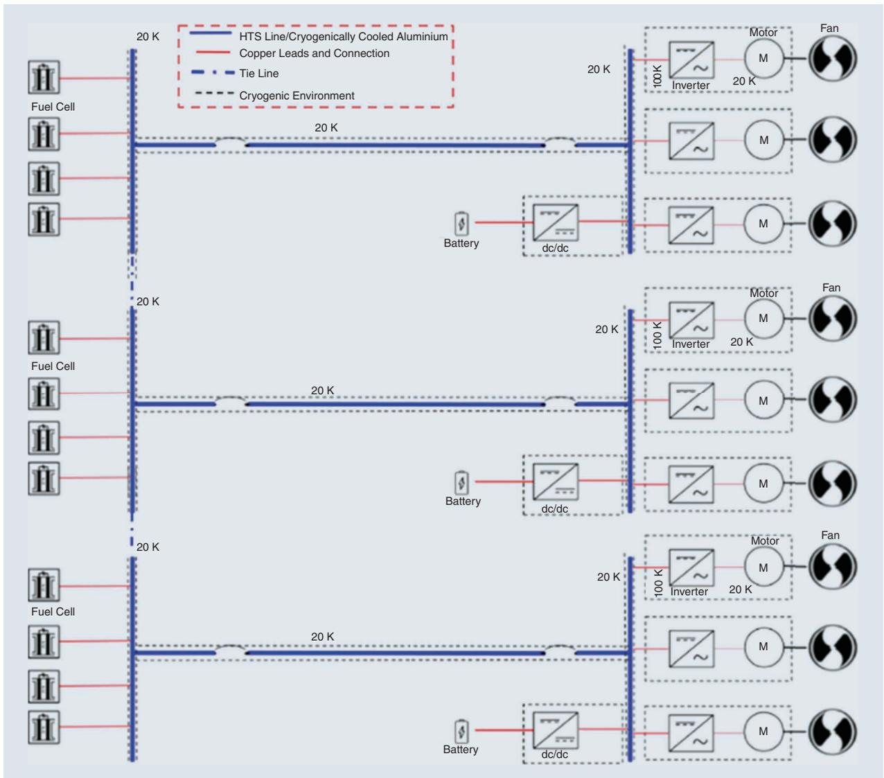
**Figure 3.** The power system architecture for a hydrogen-electric aircraft concept. HTS: high-temperature superconductor.
