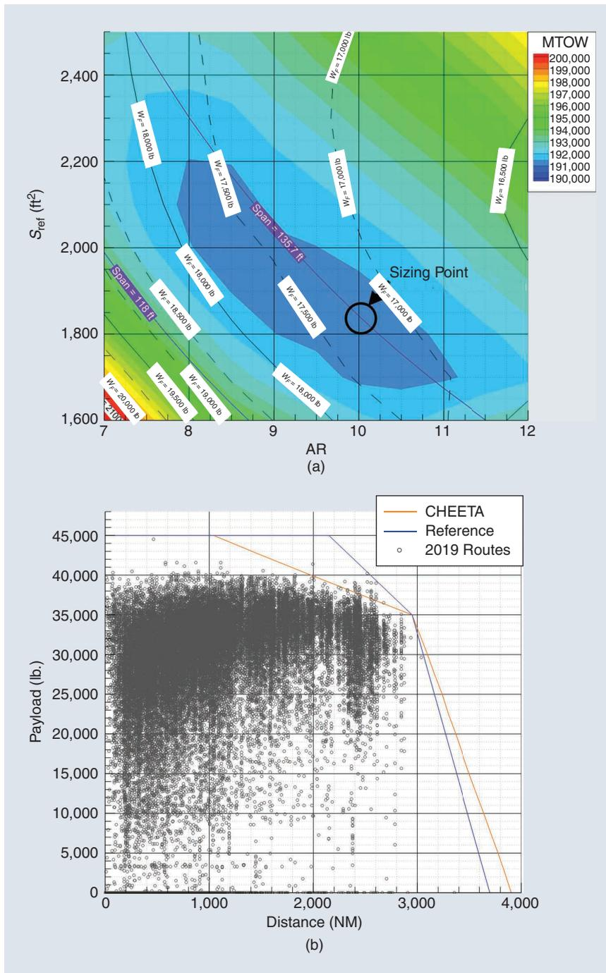
**Figure 5.** Hydrogen-electric aircraft sizing based on (a) primary wing design variables and (b) resulting payload-range capabilities.
