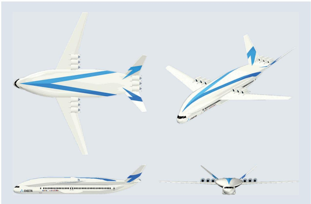
**Figure 2.** Three-view and isometric displays of a hydrogen-electric aircraft concept.
