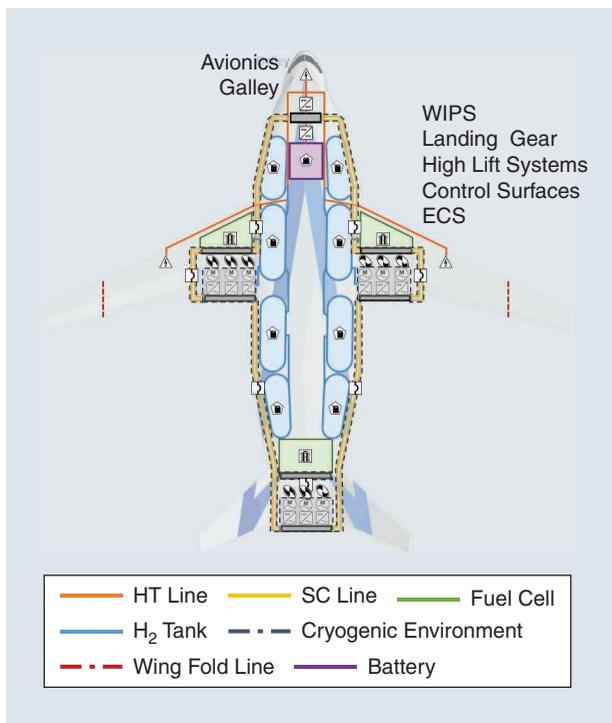
**Figure 4.** The internal layout of a hydrogen-electric power and energy system on the CHEETA configuration. ECS: Environmental Control System; HT: high temperature; SC: superconducting; WIPS: Wing Ice Protection System.
